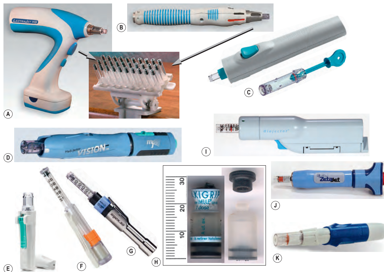
Figure 61-6 Selected Disposable-Syringe Jet Injectors (DSJIs), Licensed or Investigational (as noted). (A) Investigational LectraJet HS (high-speed) motorized DSJI (D'Antonio Consultants International 613 ) features built-in motor and rechargeable battery for rapidly compressing metal spring between injections at rates exceeding 600 per hour, with battery capacity of > 3,000 injections per charge. Capable of rapid, fingers-free loading and unloading of single-use syringes from (A, inset) a sterile-packaged, 30-unit magazine for mass vaccination. Magazine may also be mounted on nondominant forearm for vaccinator mobility. Capable of backup manual spring-cocking if batteries are depleted. (B) LectraJet M3 (manual) model DSJI, 613 sharing the same common syringe as the adjacent HS model for rapid, fingers-free loading and unloading of syringes. IM or SC delivery set by varying syringe orifice diameter. Cocked using off-tool carrying case (not shown). Cleared for US marketing by FDA in 2009. Syringes and needle-free vial adaptors also supplied in individually wrapped sterile envelopes for routine immunization (not shown). (C) PharmaJet Stratis 62 DSJI, for 0.5-mL dose delivery. Delivery IM or SC set by vaccinator technique (fat layer pinched up for SC). Cocked using off-tool carrying case (not shown). (C, inset) Syringe is filled by pulling back and breaking off its blue shaft and thumb tab from conventional single-dose and multidose vials using needle-free vial adaptor (not shown). On insertion into device, any excess liquid is returned to vial to minimize wastage of overfill. Cleared for US marketing by the FDA in 2011. See Figure 61-2J for intradermal DSJI from same device manufacturer. (D) Medi-Jector Vision DSJI, 731 used primarily for self-administration by patients of insulin and other medications. (E) Sumavel DosePro single-use DSJI (Zogenix 734 ), licensed as drug-device combination product for subcutaneous delivery of prefilled sumatriptan for treatment of migraine and cluster headaches. 735 Uses novel, borosilicate-glass dose chamber prefilled by drug manufacturer. (F) J-Tip, single-use DSJI, 733 powered by compressed nitrogen gas. (G) Injex DSJI, 732 metal spring compressed by separate cocking device. (H) Imule manufacturer-prefilled DSJI syringe 660,737 for Vaxigrip influenza vaccine (Institut Mérieux/Pasteur Mérieux Sérums & Vaccins 736 ). The syringe served as both primary vaccine packaging in a presentation smaller than conventional single-dose glass vial (millimeter scale on left), as well as the single-use disposable syringe for jet injection. Upon removing the label (H, center), inserting into the Mini-Imojet DSJI (not shown), and removing the rubber cap (H, right), the dose was ready for injection. Studied in human trials for five vaccines 134,648,650 and found successful in immune responses and safety. Subsequently abandoned by the manufacturer. (I) Biojector 2000 DSJI (Bioject Medical Technologies 83 ), capable of subcutaneous and intramuscular injections using syringes of differing orifice diameters. 614 Cleared for US marketing by FDA in 1990s. Powered by compressed CO 2 cartridge, or by connection to separate compressed gas source. An investigational spacer for intradermal delivery (illustrated elsewhere 22 ) creates a 2-cm air gap to weaken the jet stream, leaving the injectate in the skin. Used by US Navy and Coast Guard for approximately one-third million vaccinations per year of sailors and dependents from 1997 through 2011. (J) ZetaJet metal-spring-powered DSJI, 83 features built-in crank for manual re-cocking of metal spring (Bioject Medical Technologies 83 ). Uses different auto-disabling cartridges for SC, IM, and ID injections (licensed by US FDA in 2009). See Figure 61-2K for intradermal DSJI from same device manufacturer. (K) Investigational Iject DSJI, 83,730 designed for either single-use or reuse upon refitting with its manufacturer-prefilled borosilicate glass dose chamber. (Figure 61-6A, A inset, B, courtesy of D'Antonio Consultants International, Inc. 613 ; 6C, C inset, courtesy of PharmaJet, Inc. 62 ; 6D, courtesy of Antares Pharma 731 ; 6E, courtesy of Zogenix 734 ; 6F, courtesy of National Medical Products 733 ; 6G, courtesy of INJEX-Equidyne Systems 732 ; 6H, courtesy of Bruce G. Weniger; 6I, courtesy of James Gathany (CDC Photographic Services); 6J, K, courtesy of Bioject Medical Technologies. 83 )
